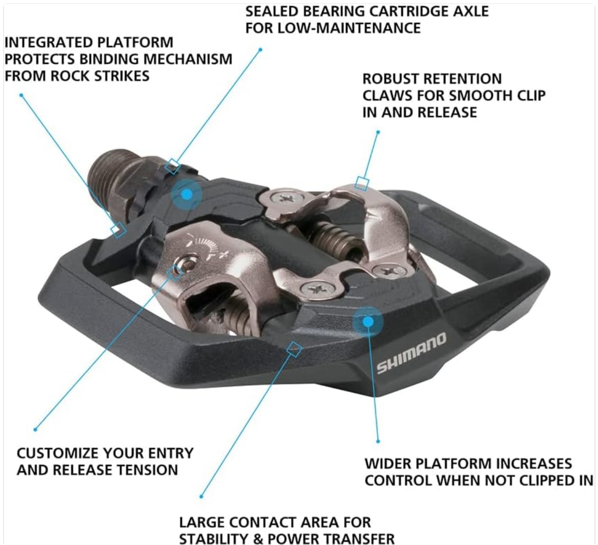
Figure 2: Key features of the PD-ME700 Pedals, highlighting the integrated platform, sealed bearing cartridge axle, robust retention claws, customizable tension, and wider platform for increased control.
