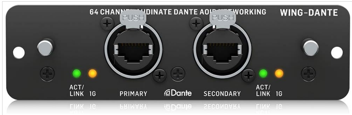
Figure 1: Front view of the Behringer WING-DANTE expansion card. Shows two Ethernet ports labeled 'PRIMARY' and 'SECONDARY', each with 'ACT/LINK 1G' status LEDs. The card is black with white text.
