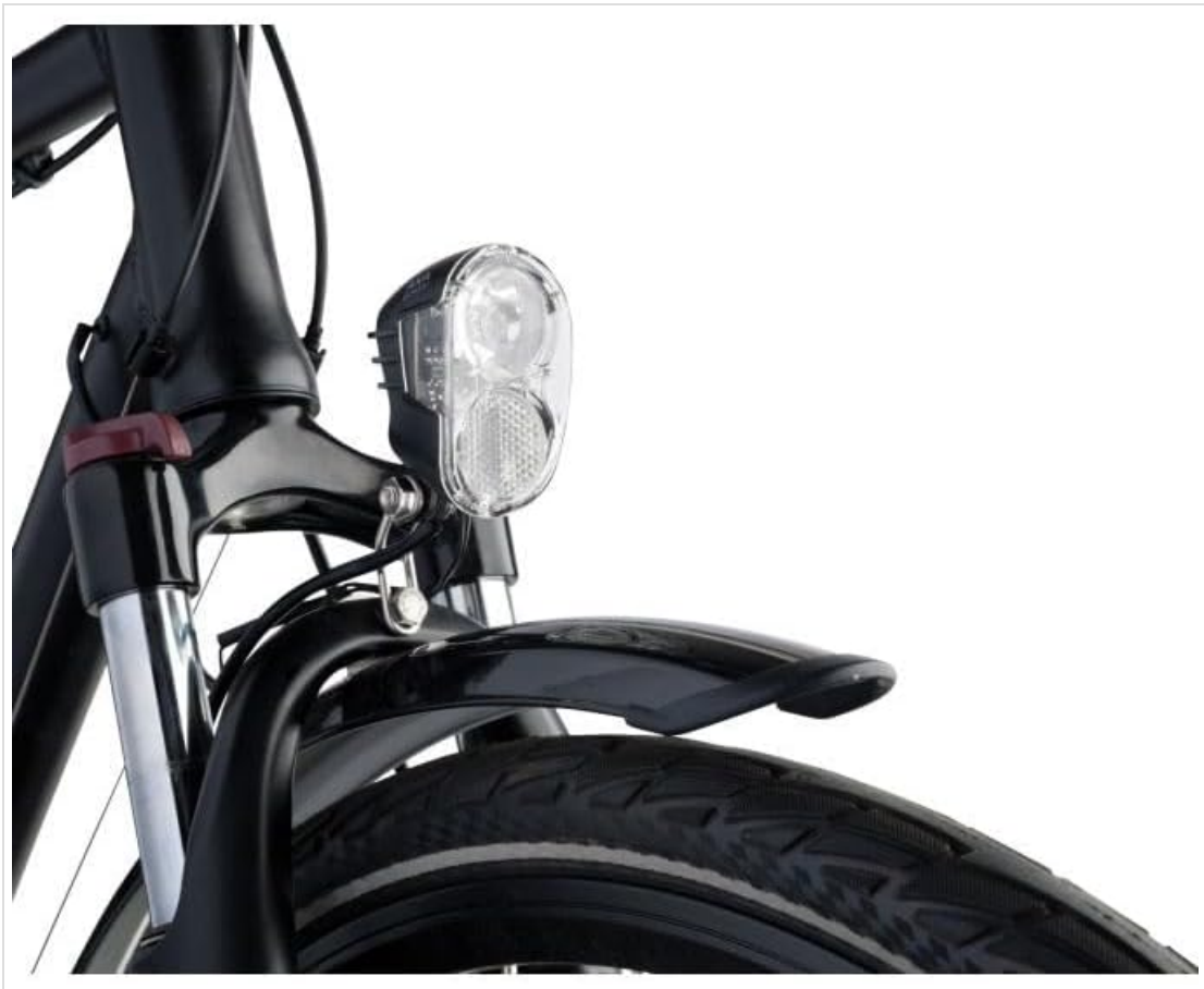
Image 3.1: The AXA Echo 15 Headlight correctly mounted on the front fork of a bicycle.
