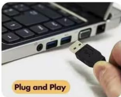
Figure 2: Simple two-step setup: Plug the webcam's USB cable into your computer and open your desired software to begin use.
