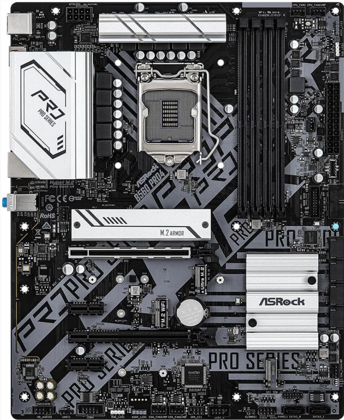
Figure 1: Top-down view of the ASRock B560 PRO4 motherboard, highlighting the CPU socket, RAM slots, PCIe slots, and M.2 heatsinks.
