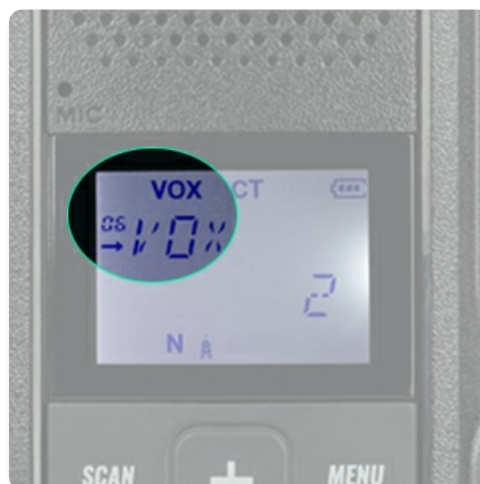
Image 4.5: Retevis RB27 VOX Feature. This image displays the radio's screen indicating the VOX function is active, enabling voice-activated transmission.
