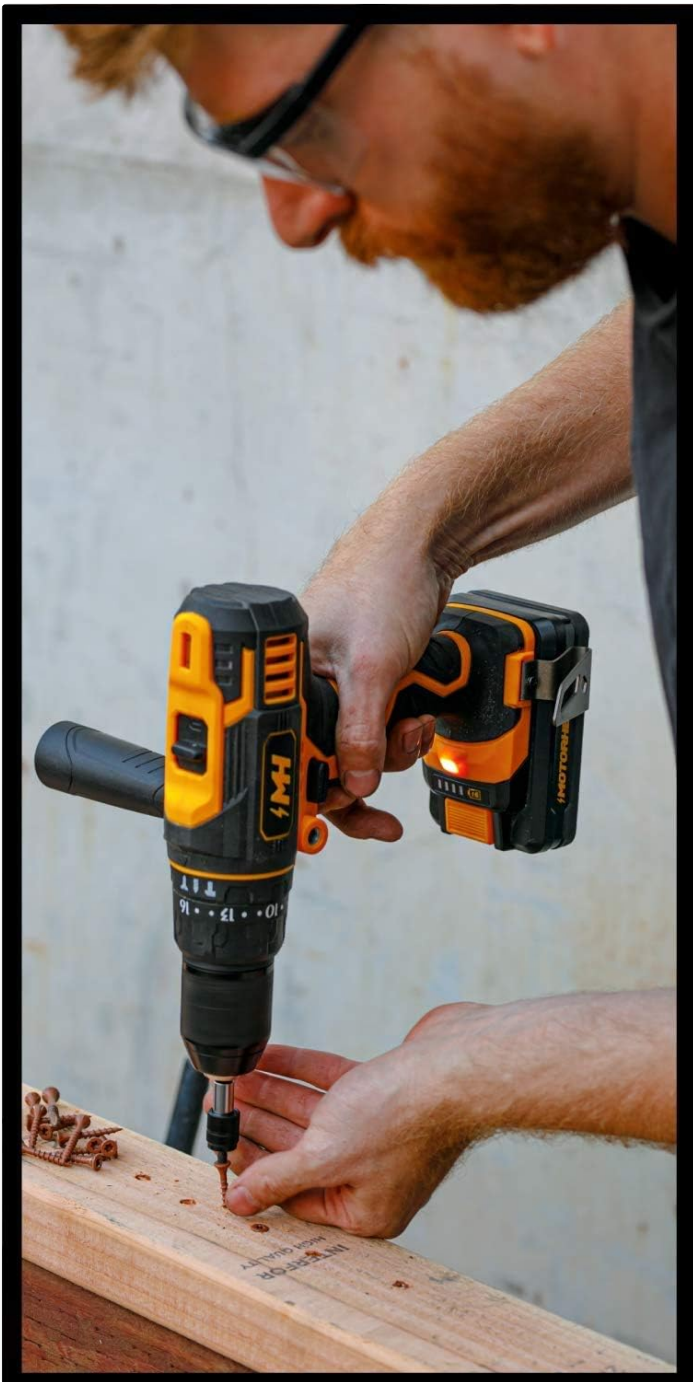
Image 6.1: Driving a screw into a wooden surface with the drill driver.
