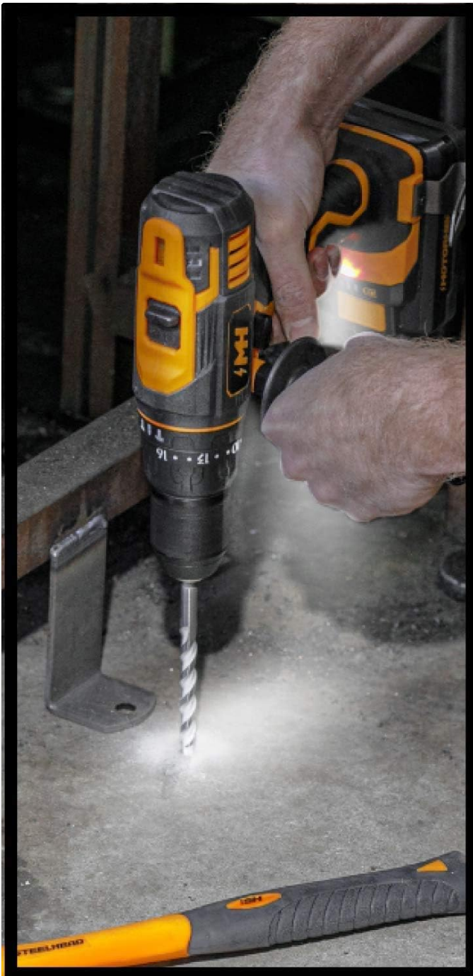
Image 6.2: Using the hammer drill function on concrete and drilling into metal.
