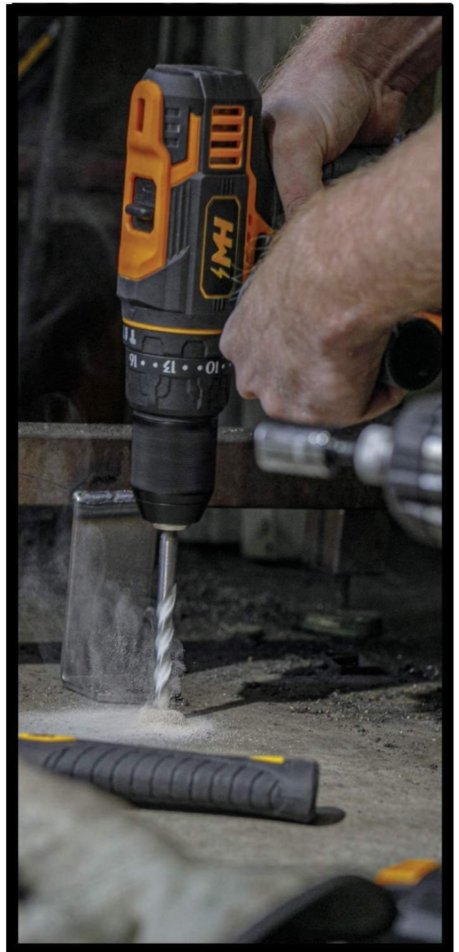
Image 6.2: Using the hammer drill function on concrete and drilling into metal.
