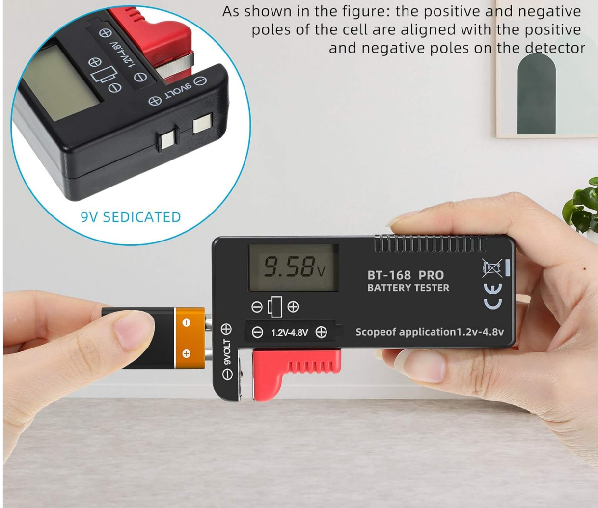
Figure 5: A 9V battery being tested by connecting its terminals to the dedicated 9V contacts on the BT-168 PRO tester, with the voltage displayed on the screen.
