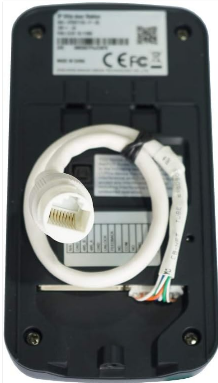
Figure 4.1: Rear view of the Dahua VTO2111D-P-S2 IP Villa Doorbell with an Ethernet cable connected, illustrating the wiring process.
