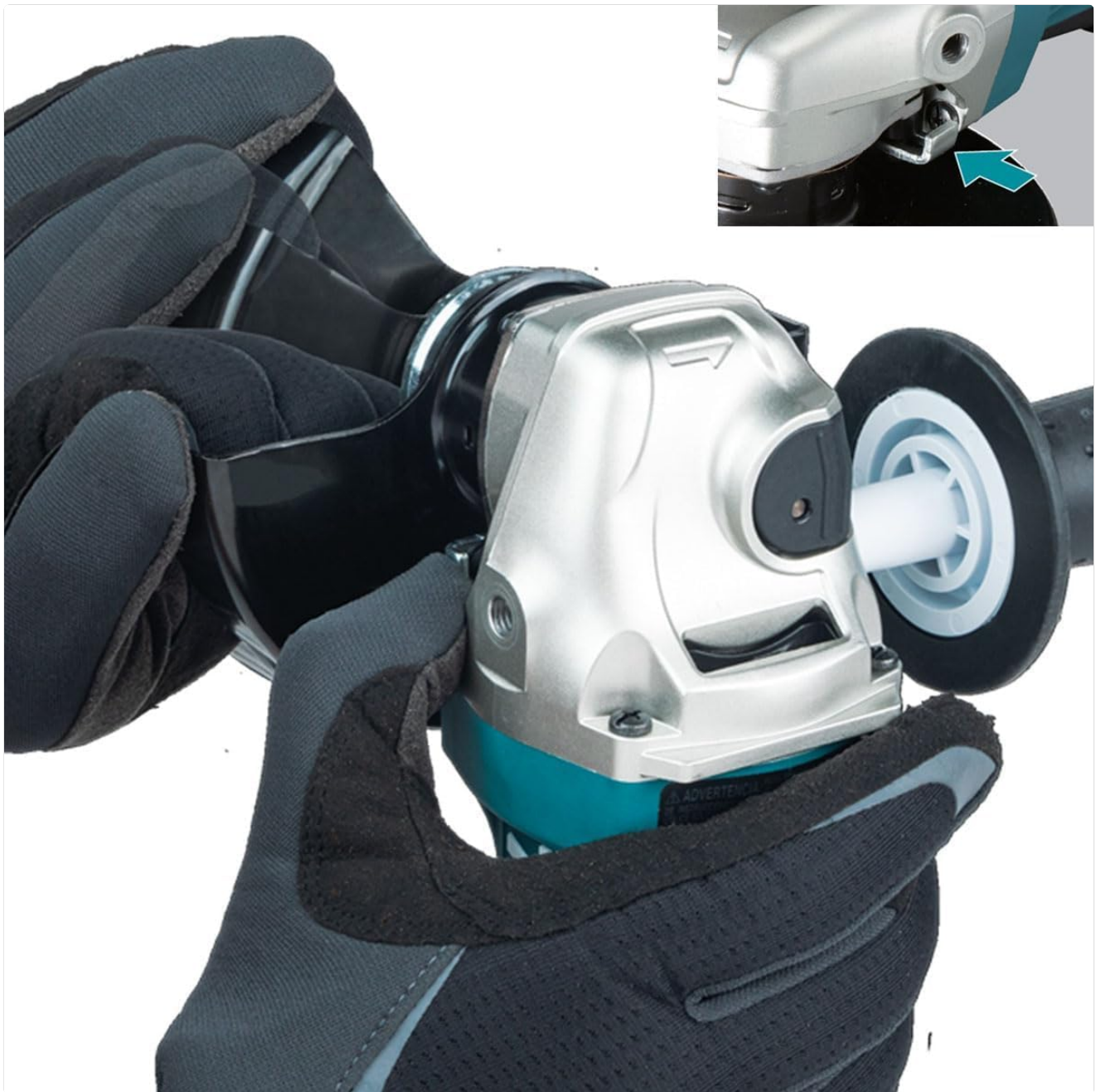
Figure 6: Hands demonstrating the adjustment of the wheel guard. The inset shows a close-up of the guard's locking lever or screw for secure positioning.
