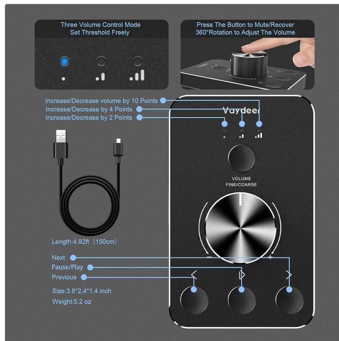
Image 2.2: A detailed diagram illustrating the three volume control modes (2, 4, or 10 points per step) and the functions of the play/pause and track skip buttons.
