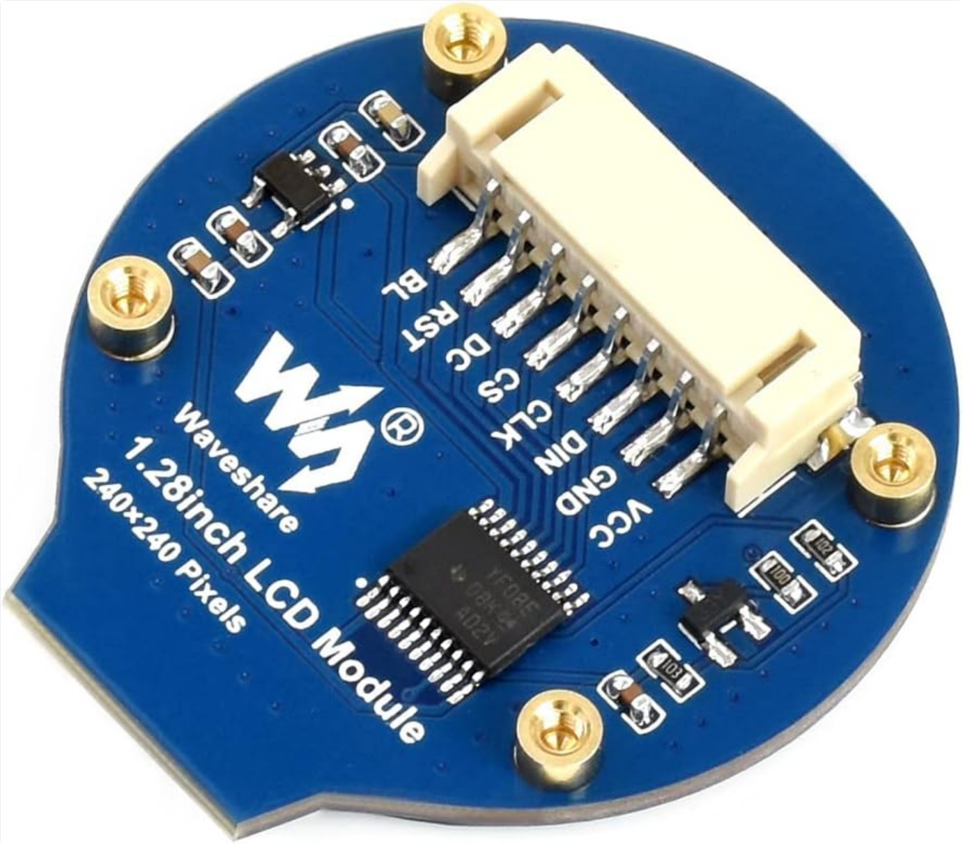
Figure 4: Back view of the display module showing the 8-pin connector and pin labels.
