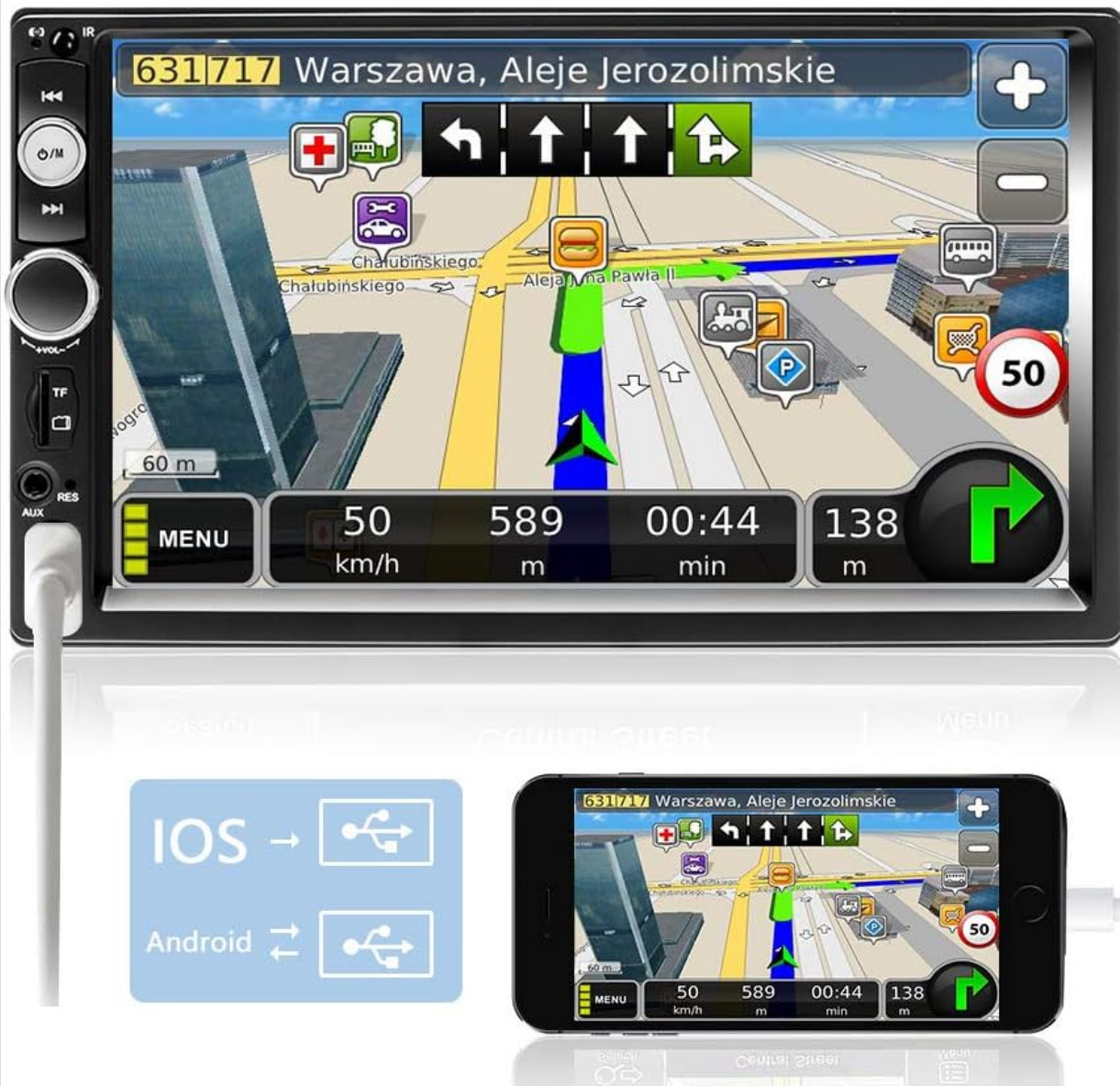
Figure 5.3: Mirror Link in action, showing a GPS navigation application from a connected smartphone mirrored onto the car stereo display.
