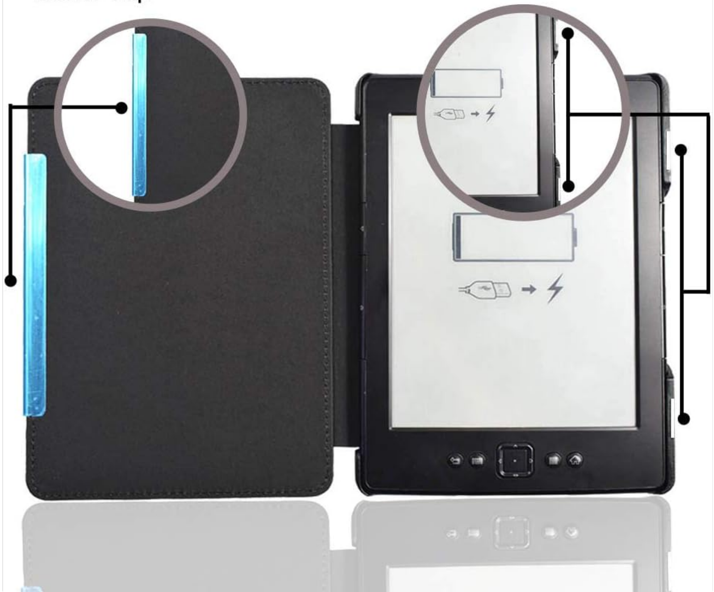
Figure 3: Magnetic Clasp Mechanism. A metal clip and integrated magnets ensure the cover stays closed, protecting the screen.
