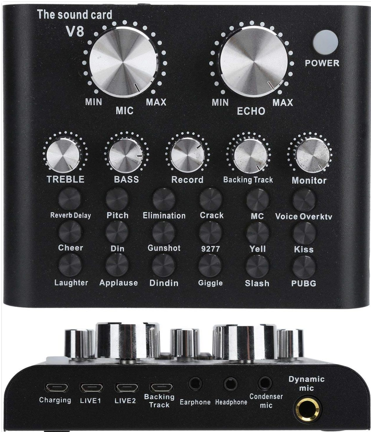
Figure 4.3: Bottom view of the Lazmin112 V8 Sound Mixer Board, illustrating the Charging port, LIVE1, LIVE2, Backing Track, Earphone, Headphone, Condenser mic, and Dynamic mic ports.
