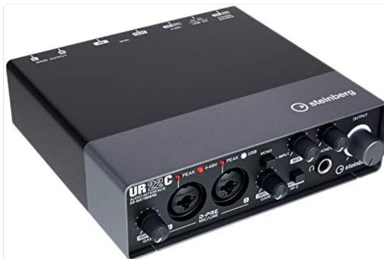
Figure 4.2: Front panel of the UR22C with input jacks and control knobs.
