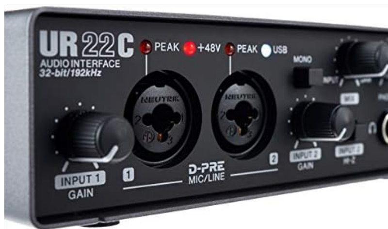
Figure 5.1: Close-up of input gain controls and PEAK indicators.
