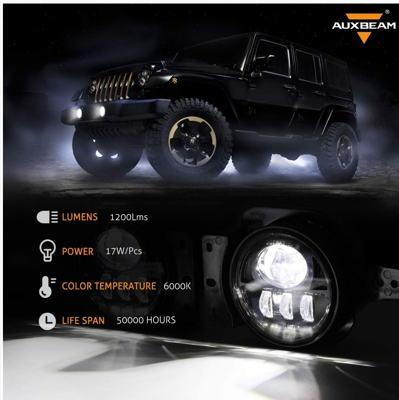
Figure 2: Key specifications of the fog lights, including 1200 lumens, 17W/Pcs, 6000K color temperature, and 50,000 hours lifespan.
