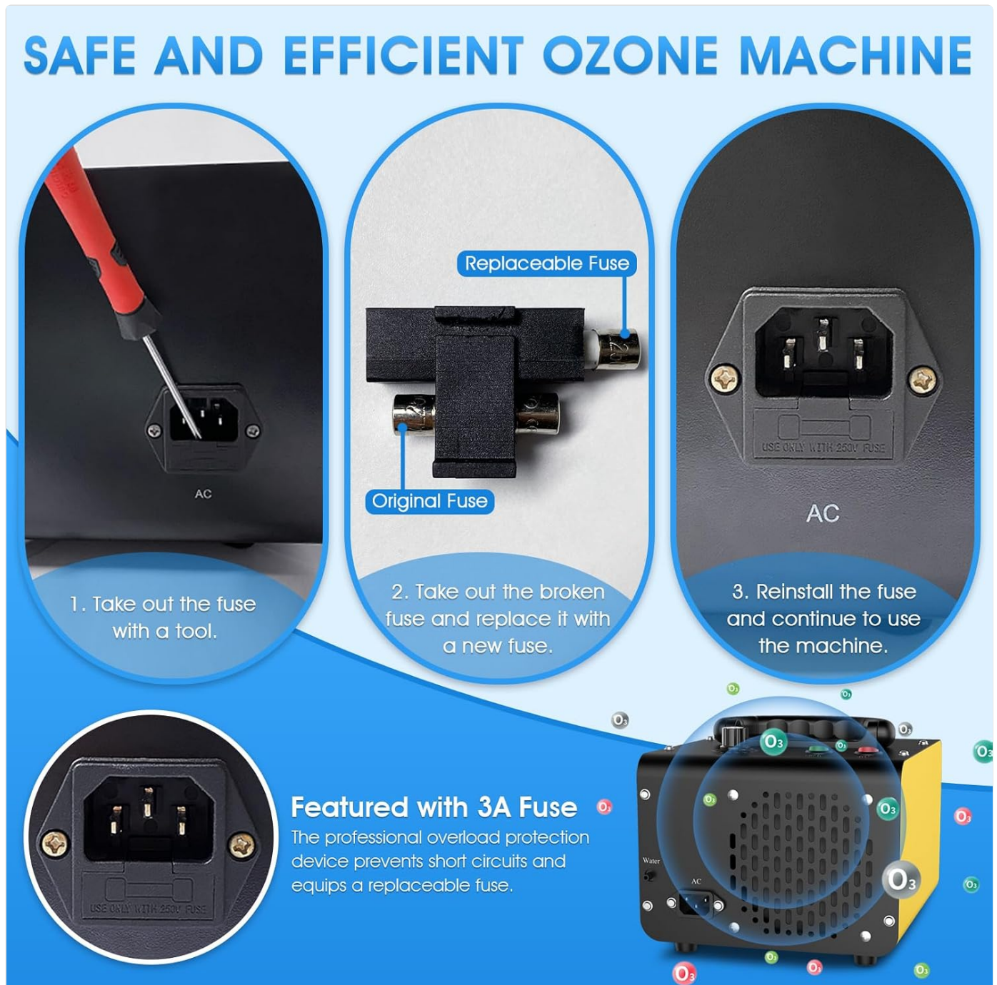
Figure 7: Steps for replacing the fuse.
