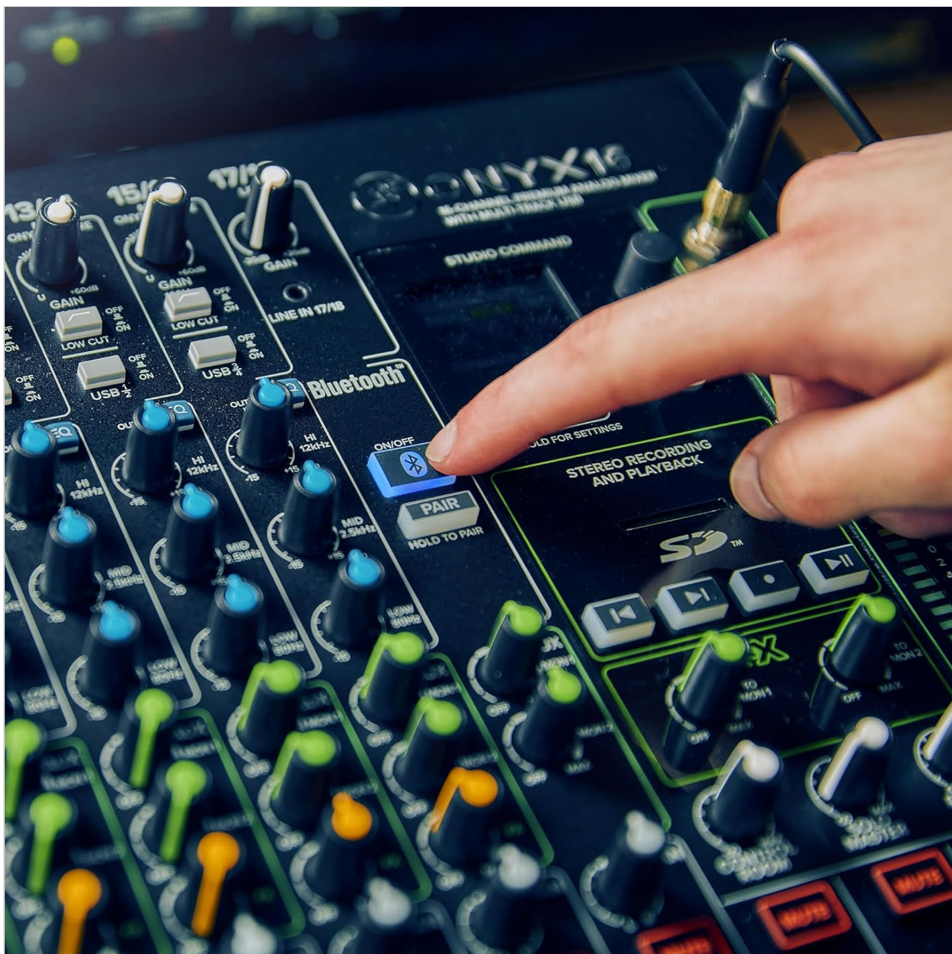
Figure 4: Close-up of the Studio Command section, showing Bluetooth pairing controls and SD card recording/playback buttons.
