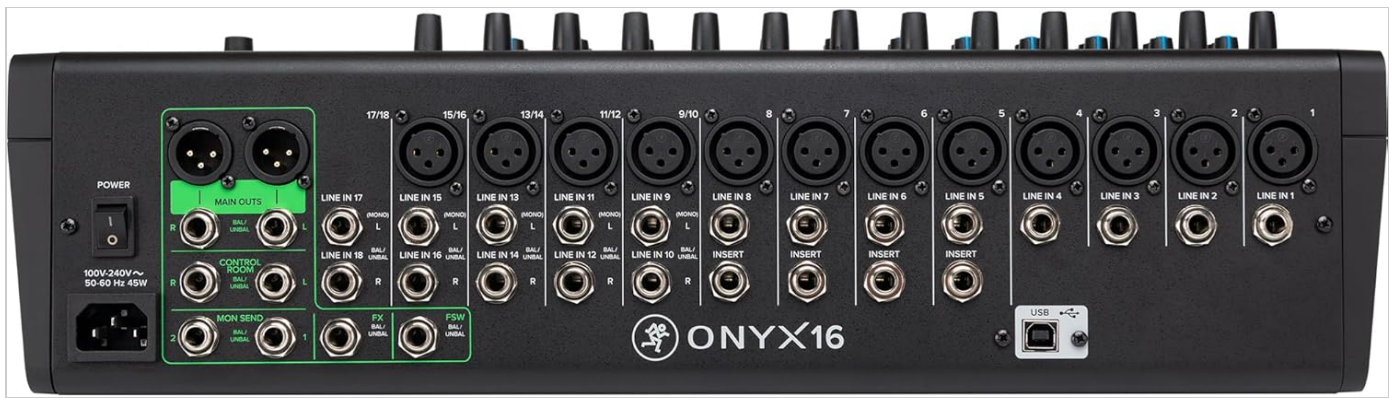
Figure 2: Rear panel view of the Mackie Onyx16 mixer, detailing the various input and output connectors including XLR, 1/4" TRS, and USB.
