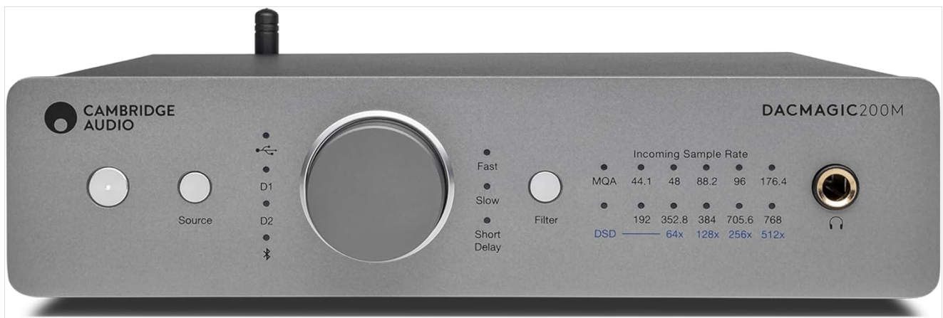
Front panel of the Cambridge Audio DacMagic 200M, showing input selection, volume knob, filter selection, sample rate indicators, and headphone jack.
