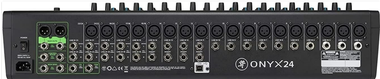
Figure 3.1: Rear panel of the Mackie Onyx24, showing input/output connections and power input.
