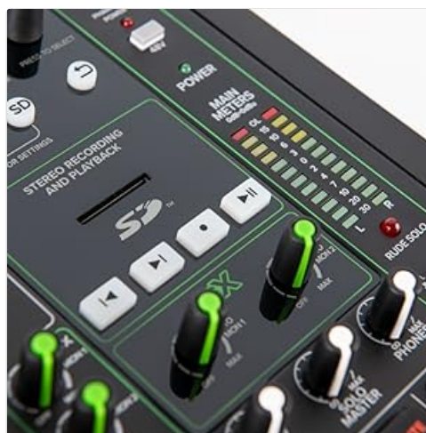
Figure 3.2: Close-up of the SD card recording and playback controls on the Onyx24.
