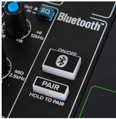
Figure 4.5: Bluetooth ON/OFF and PAIR buttons for wireless audio streaming.
