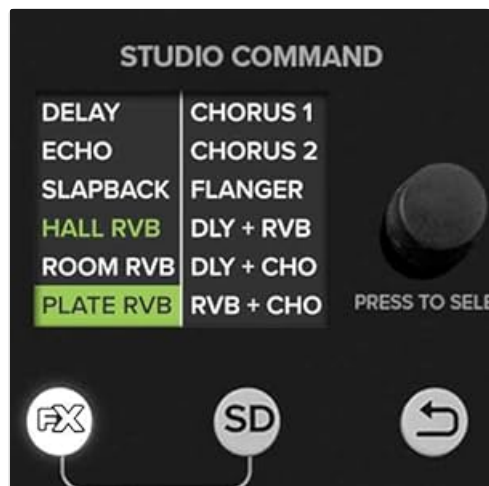
Figure 4.4: The DSP effects display and selection controls.
