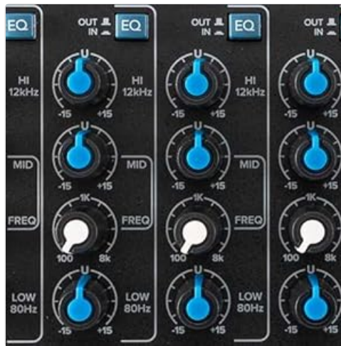
Figure 4.3: Detail of the Perkins EQ section, including High, Mid (sweepable), and Low frequency controls.
