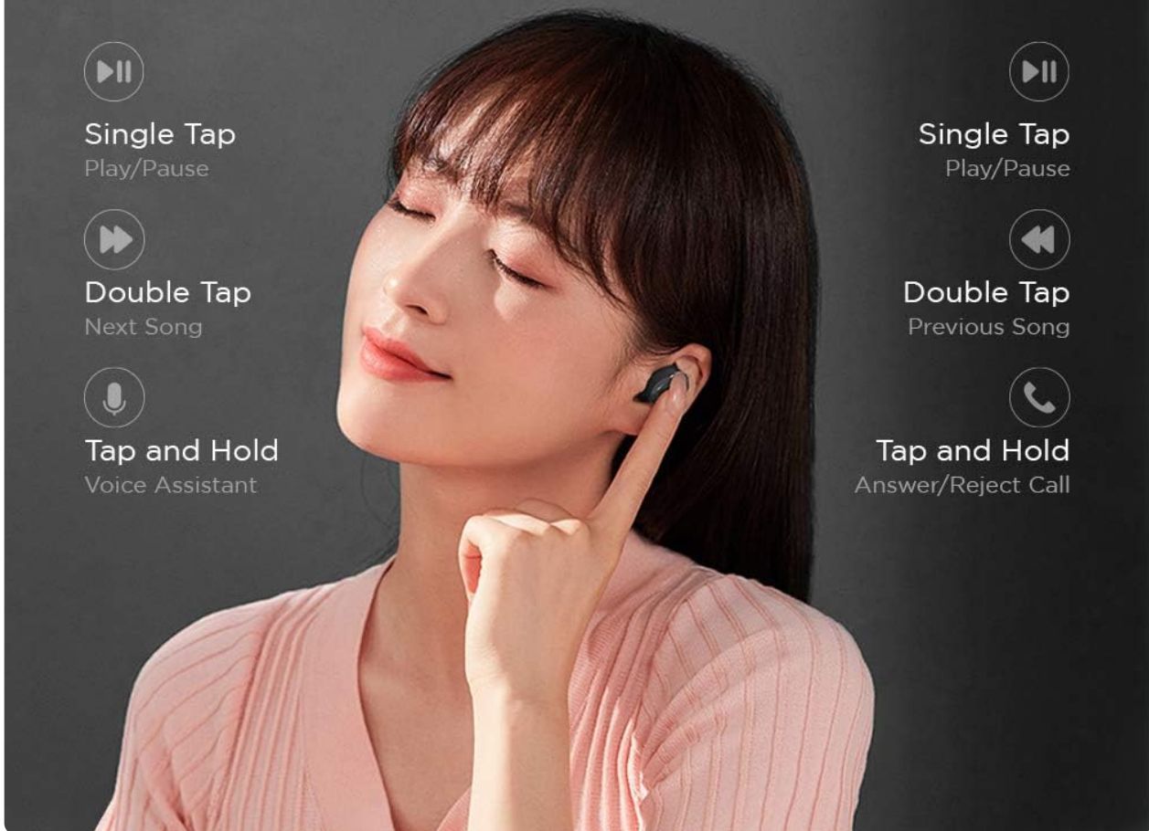
Image 4.1: Visual guide to touch controls for play/pause, next/previous song, voice assistant, and call management.
