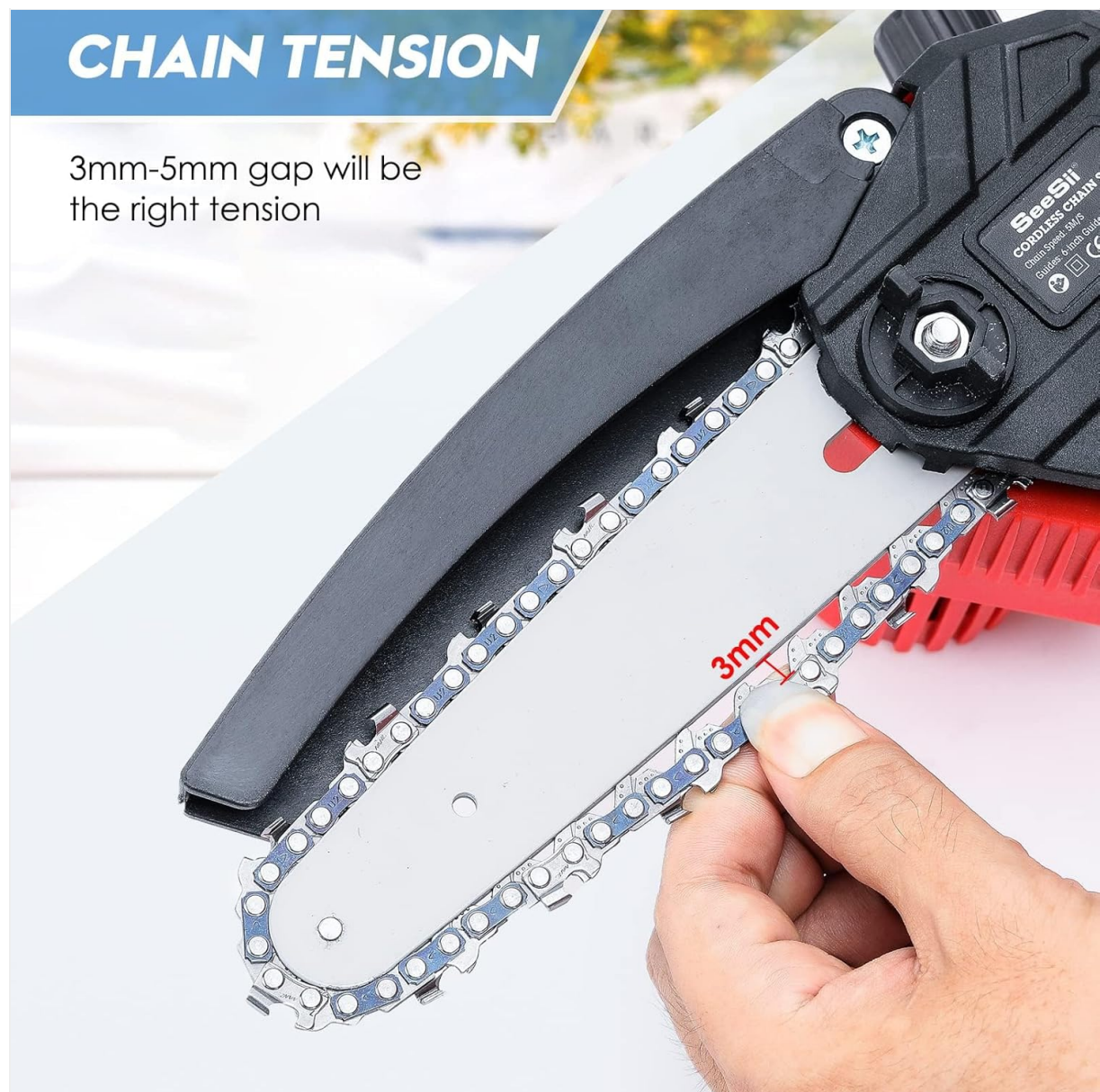
Figure 6.1: Chain Tension Check. This image illustrates the correct method for checking chain tension, aiming for a 3mm-5mm gap.
