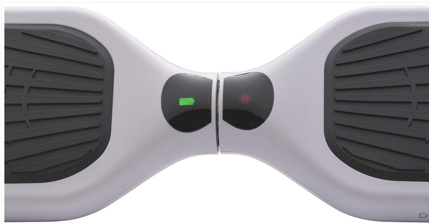
Figure 3: Central section of the hoverboard showing the battery indicator (green) and the status indicator (red), which illuminate to provide operational feedback.
