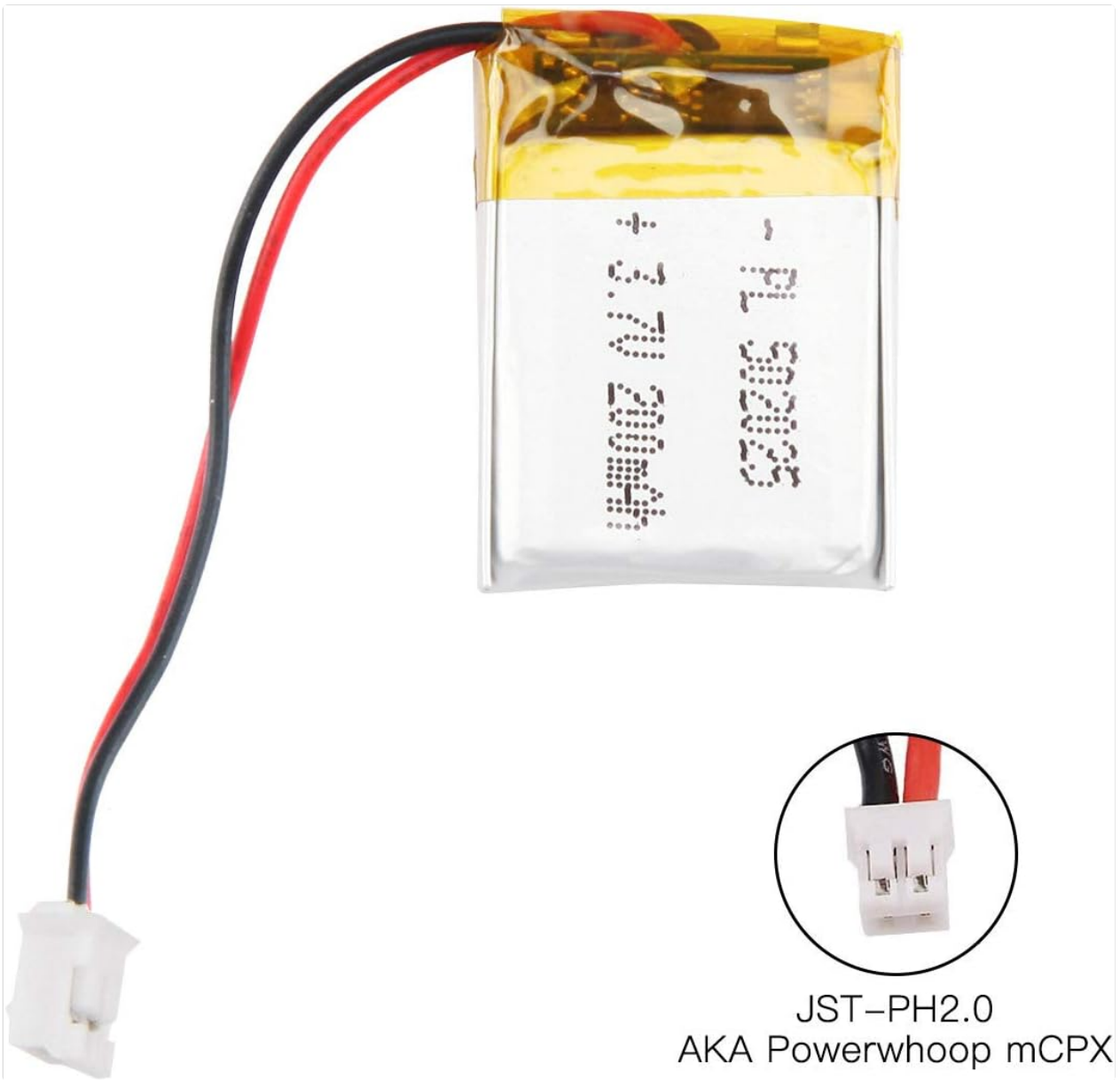
Figure 2: Detailed view of the JST-PH2.0 connector, also known as mCPX.
