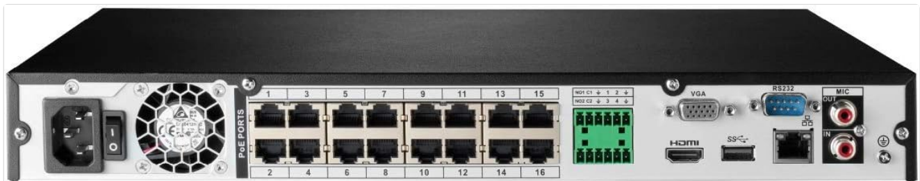
Figure 2: Lorex NVR Rear Panel. This image shows the back of the NVR unit, highlighting various ports including 16 PoE ports, HDMI, VGA, USB, Ethernet, audio input/output, and power input.
