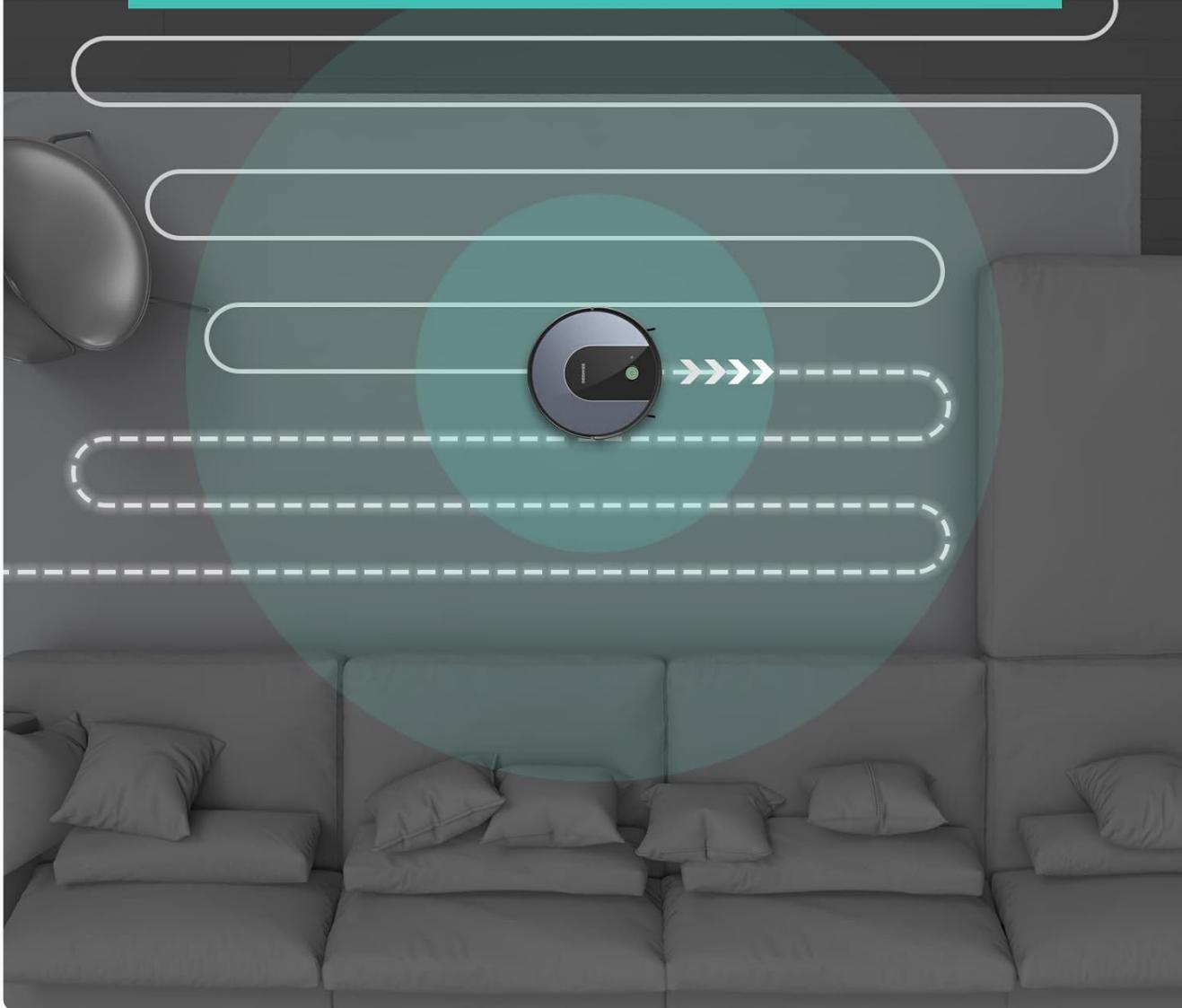
The robot vacuum employs gyroscopic navigation for systematic and efficient cleaning paths.
