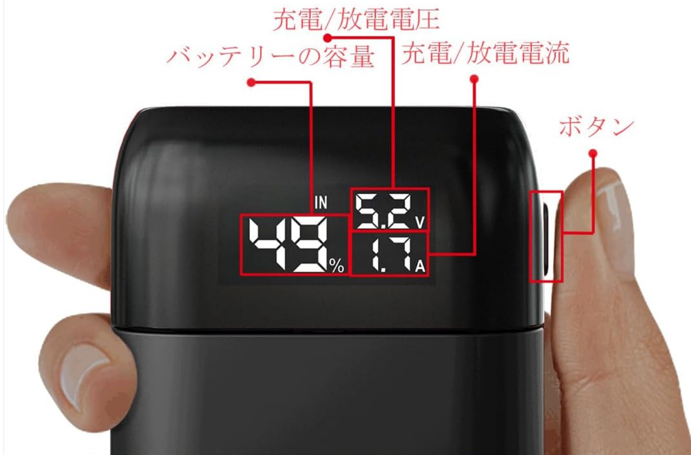
Image: The XTAR PC2's digital display indicating battery capacity percentage, voltage, and current during operation.
