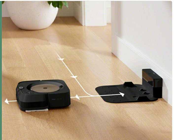
Figure 5.6: The Braava Jet m6 robot mop's Smart Charge & Resume feature, allowing it to intelligently recharge and continue cleaning until the task is complete.
