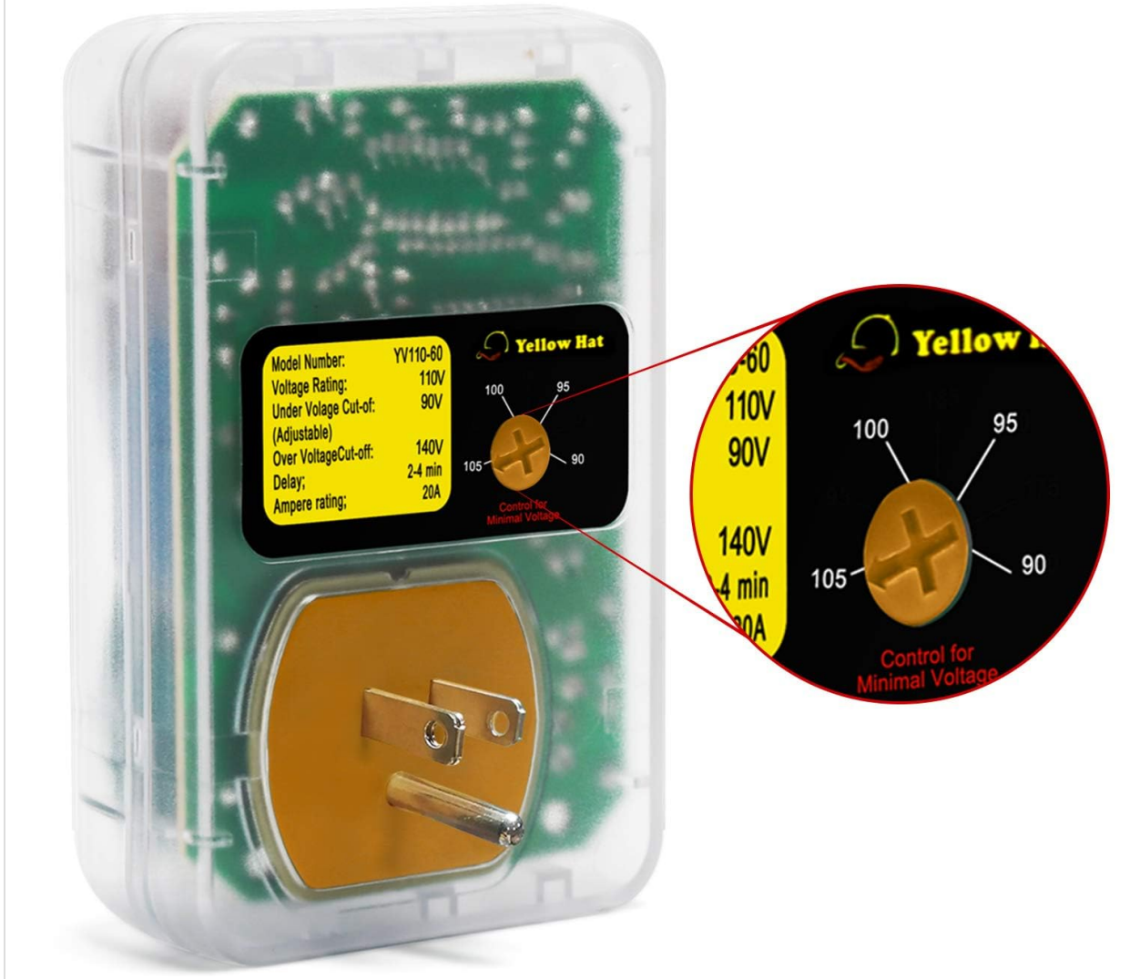
Image 6.1: The adjustable knob on the back of the surge protector allows users to set the desired minimum voltage cut-off between 90V and 140V.
