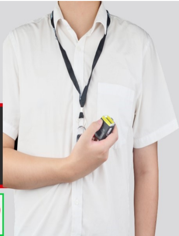
Image 4.2: A user performing NFC pairing by tapping the GS02 scanner to an Android smartphone.
