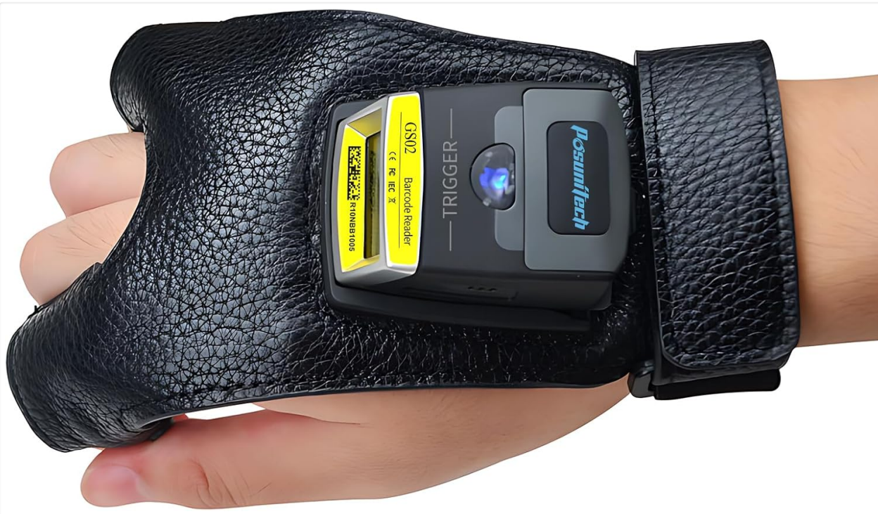
Image 1.1: The Posunitech GS02 wearable barcode scanner securely fitted on a user's hand, demonstrating its hands-free design.
