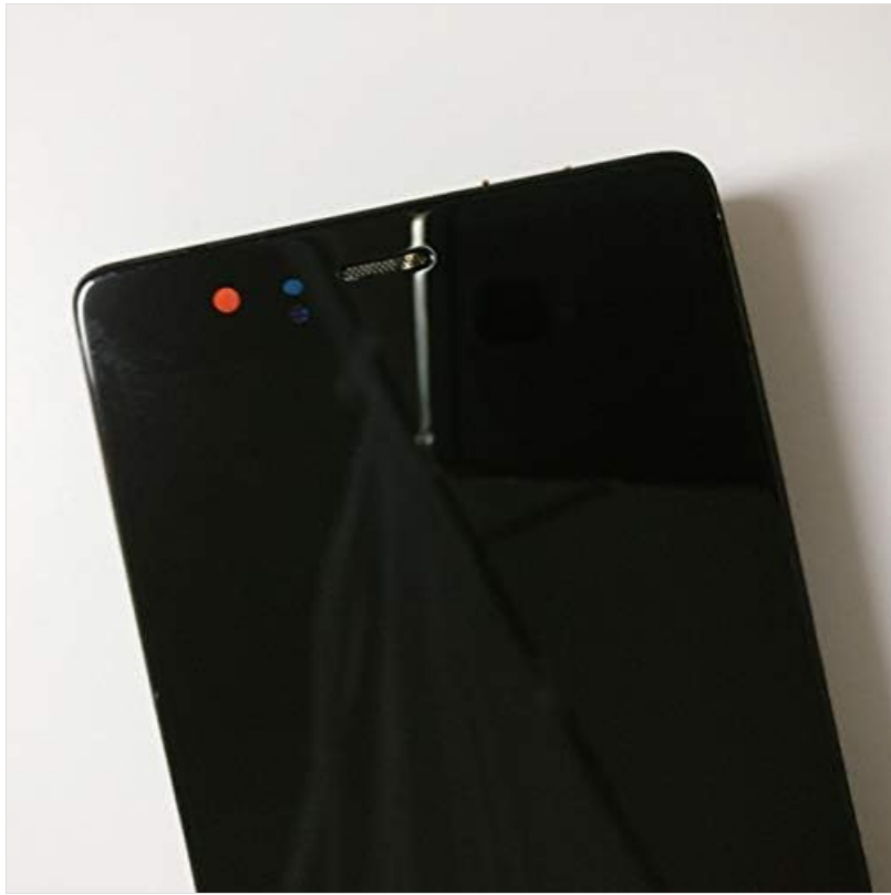
Image 3: Front view of the upper section of the Lysee Heyman LCD screen, showing the earpiece cutout and sensor areas.
