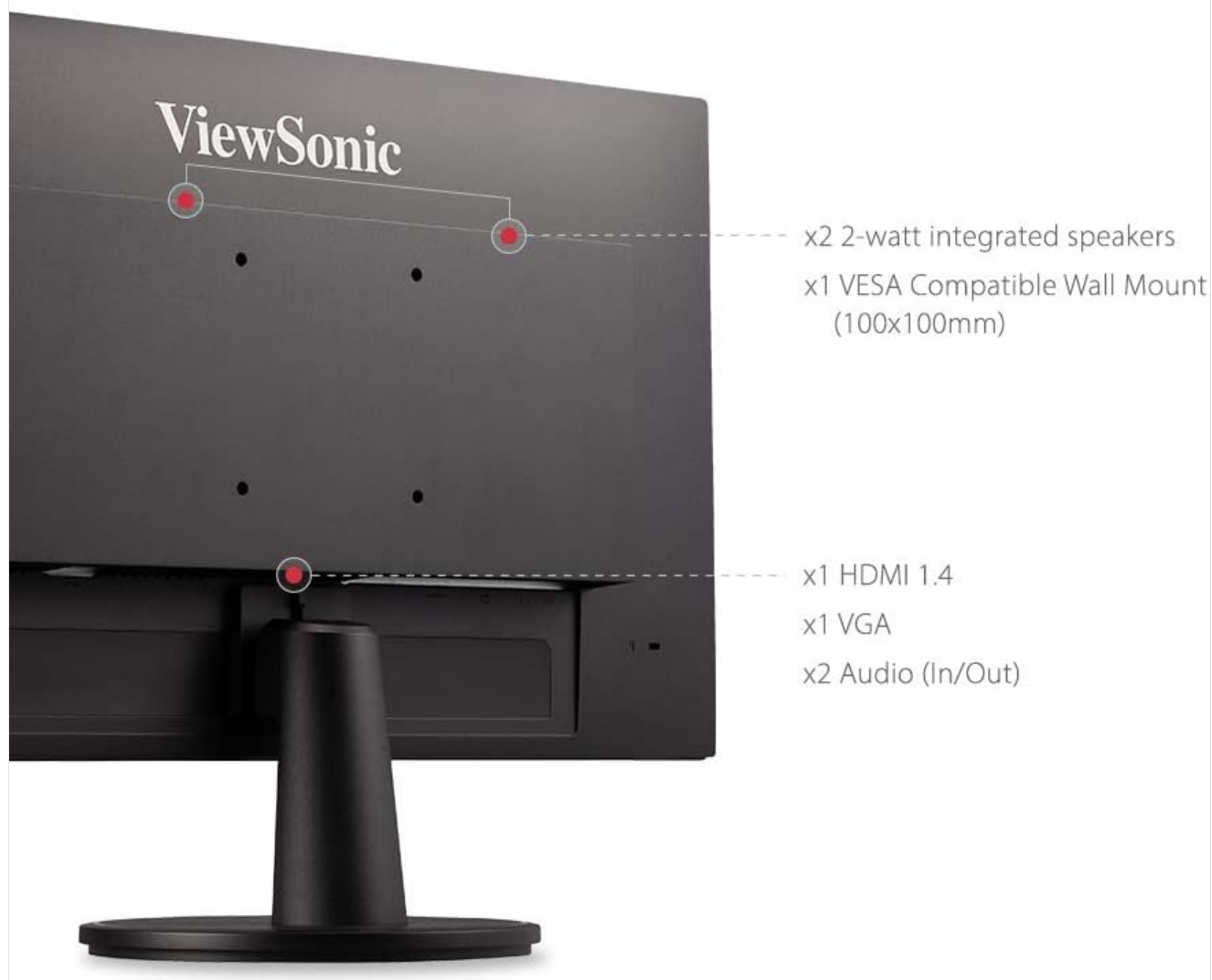
Figure 2.2: Rear panel showing HDMI, VGA, and audio input/output ports, along with integrated speakers and VESA mount points.
