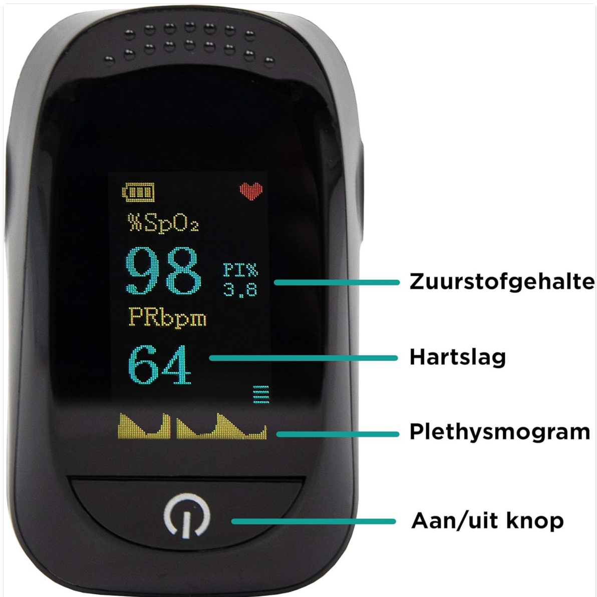
Close-up of the Silvergear Pulse Oximeter display with labels indicating Oxygen Saturation, Pulse Rate, Plethysmogram, and Power Button.
