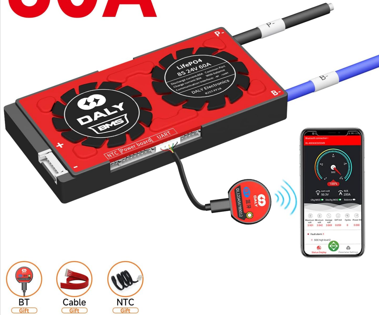
Figure 7: DALY Smart BMS connected to a smartphone app via Bluetooth for real-time monitoring.
