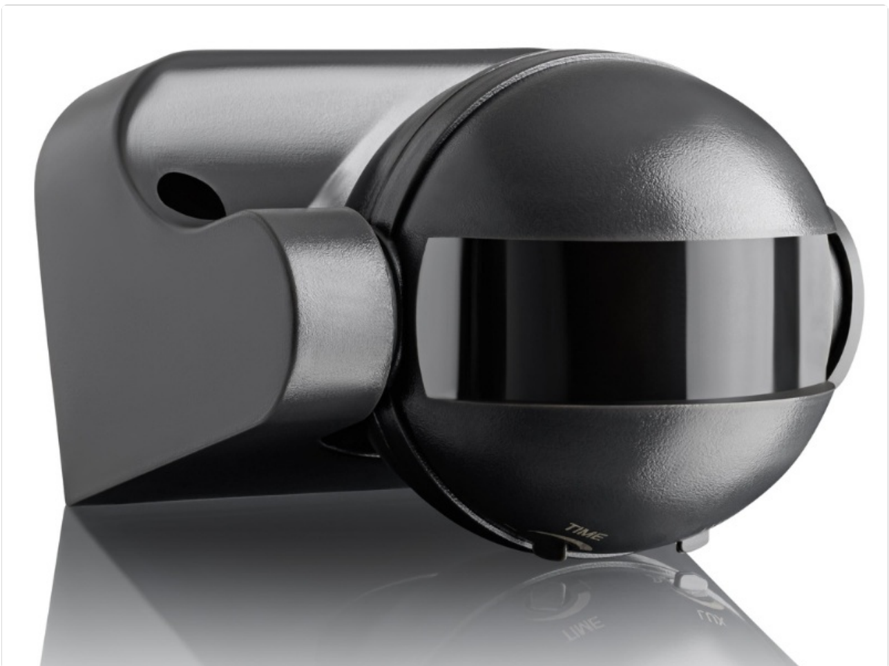
Image 4.1: Overview of key product features: 12m/180° detection, up to 300W LED, IP44 rating, 10 sec - 7 min duration, 3-2000 LUX sensitivity, 230V operation.
