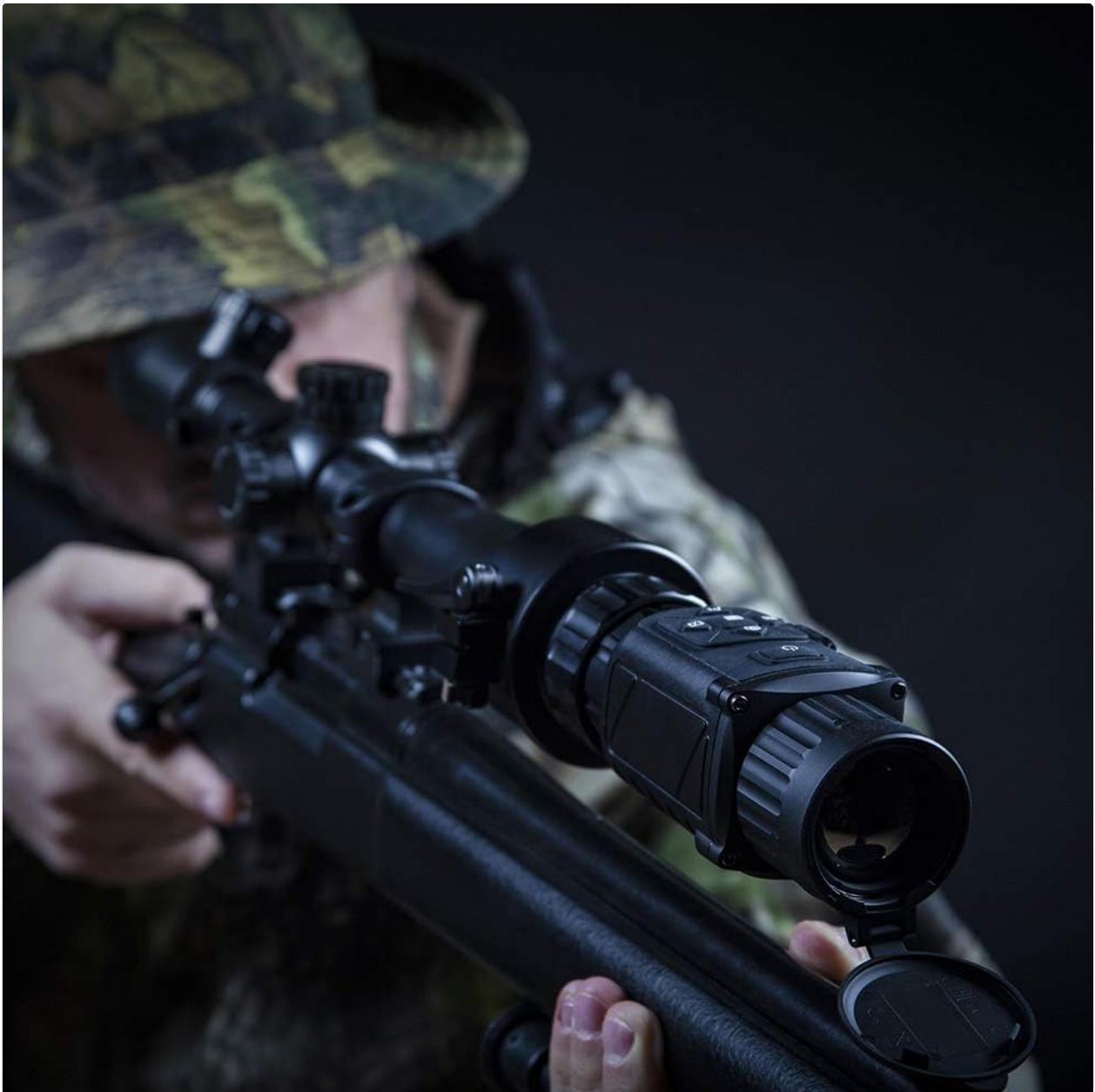
Figure 6.1: A user operating the thermal clip-on device, demonstrating its use in conjunction with a riflescope.
