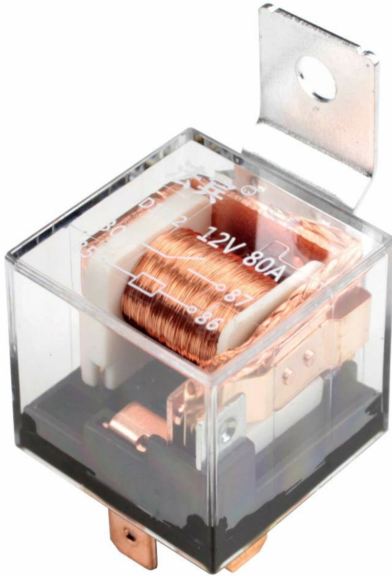
Figure 2.3: Close-up view of the 12V 80A relay, showing its transparent housing and copper coil.
