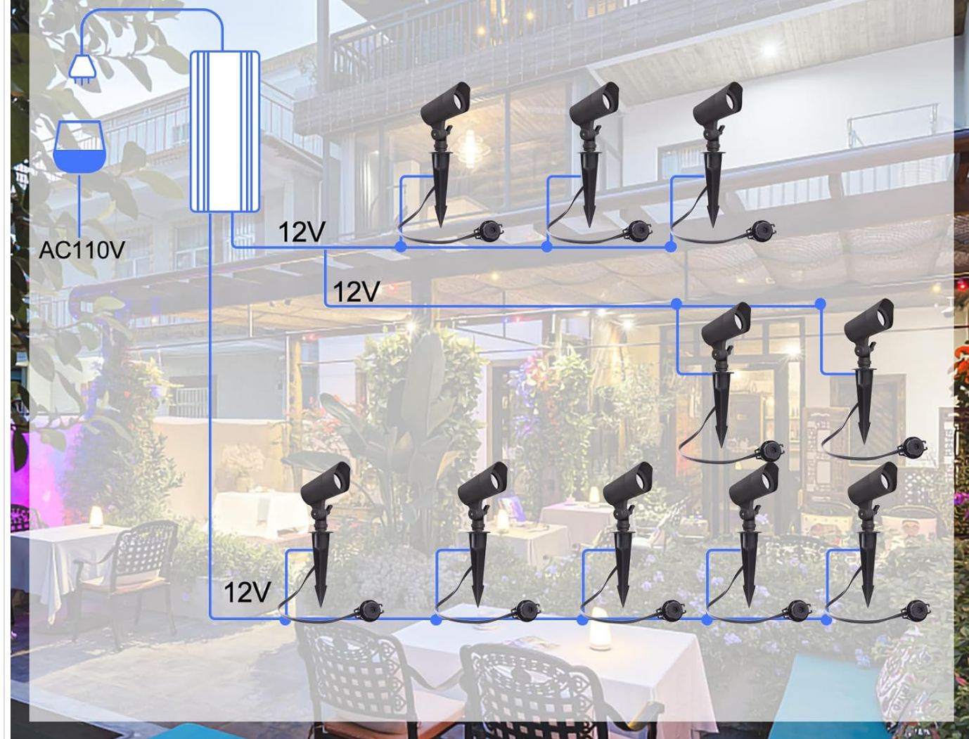
Image: An illustrative diagram of a typical low voltage LED landscape light installation layout.
