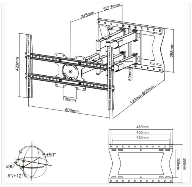
Detailed technical drawing showing the dimensions of the wall mount, including VESA compatibility and articulation points.
