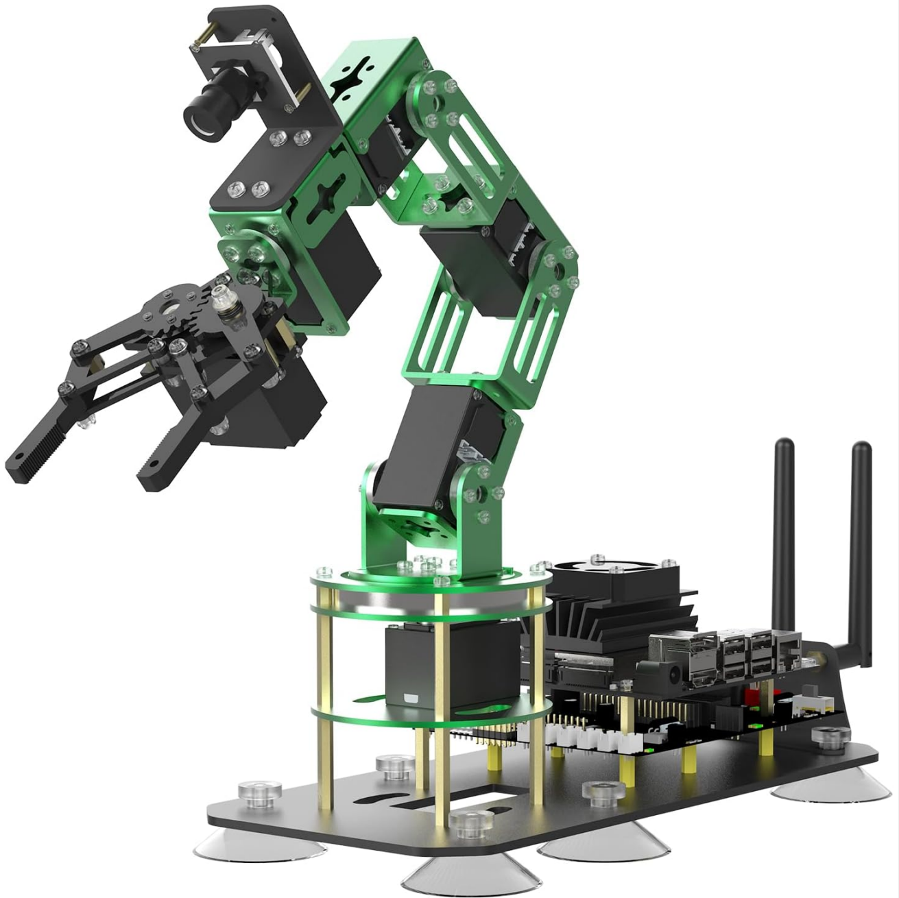
Figure 2.1: The Yahboom Nano-DOFBOT 6DOF AI Vision Robot Arm Kit, showcasing its green robotic arm, base, and integrated electronics.
