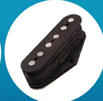
bridge P/U: Alnico 5 magnet, resistance 10k \Omega
