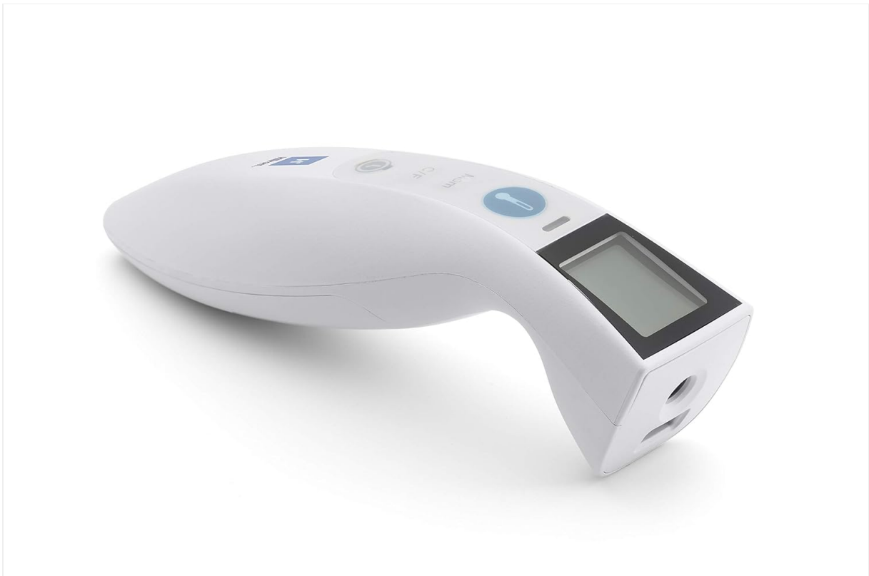
Image 3: View of the Welch Allyn Contact-Free Forehead Thermometer, highlighting the infrared sensor area at the front, which should be aimed at the forehead for accurate readings.
