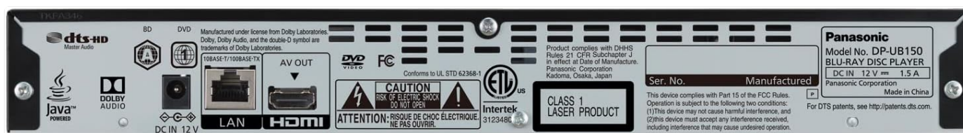
Image 4.1: Rear panel connections of the player, highlighting the HDMI, LAN, and power input ports.
