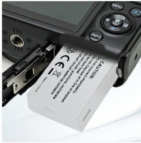
Image: Proper insertion of the LP E5 battery into a camera's battery compartment.
