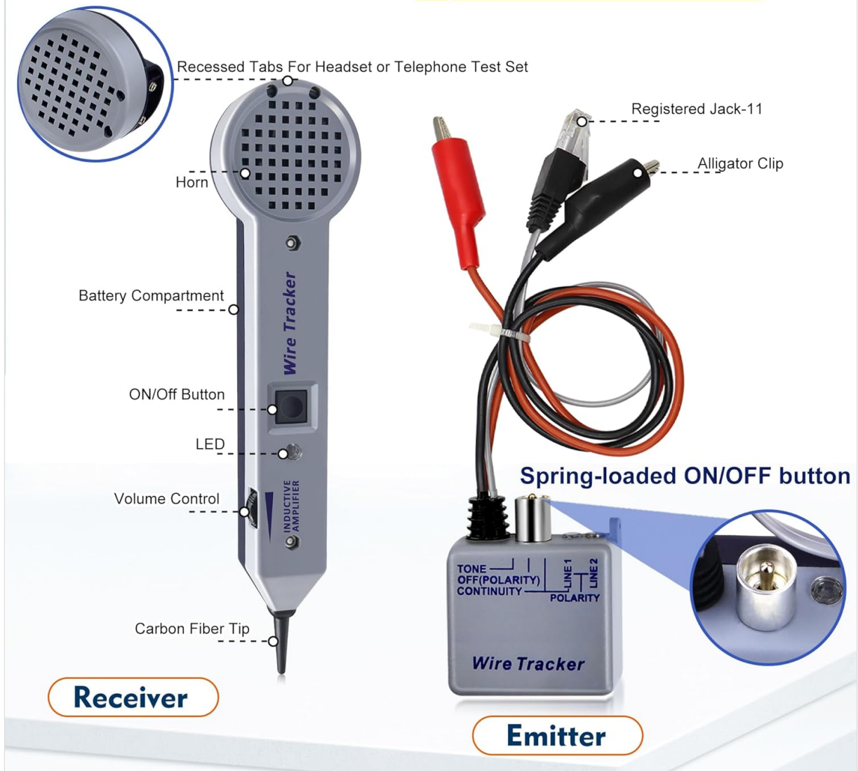
Image 3: A detailed view of the Lunarlipos 200EP Tone Generator (Emitter) and Inductive Amplifier (Receiver), highlighting key features such as the horn, battery compartment, ON/OFF button, LED indicator, volume control, carbon fiber tip on the receiver, and the registered Jack-11, alligator clips, and spring-loaded ON/OFF button on the emitter.
