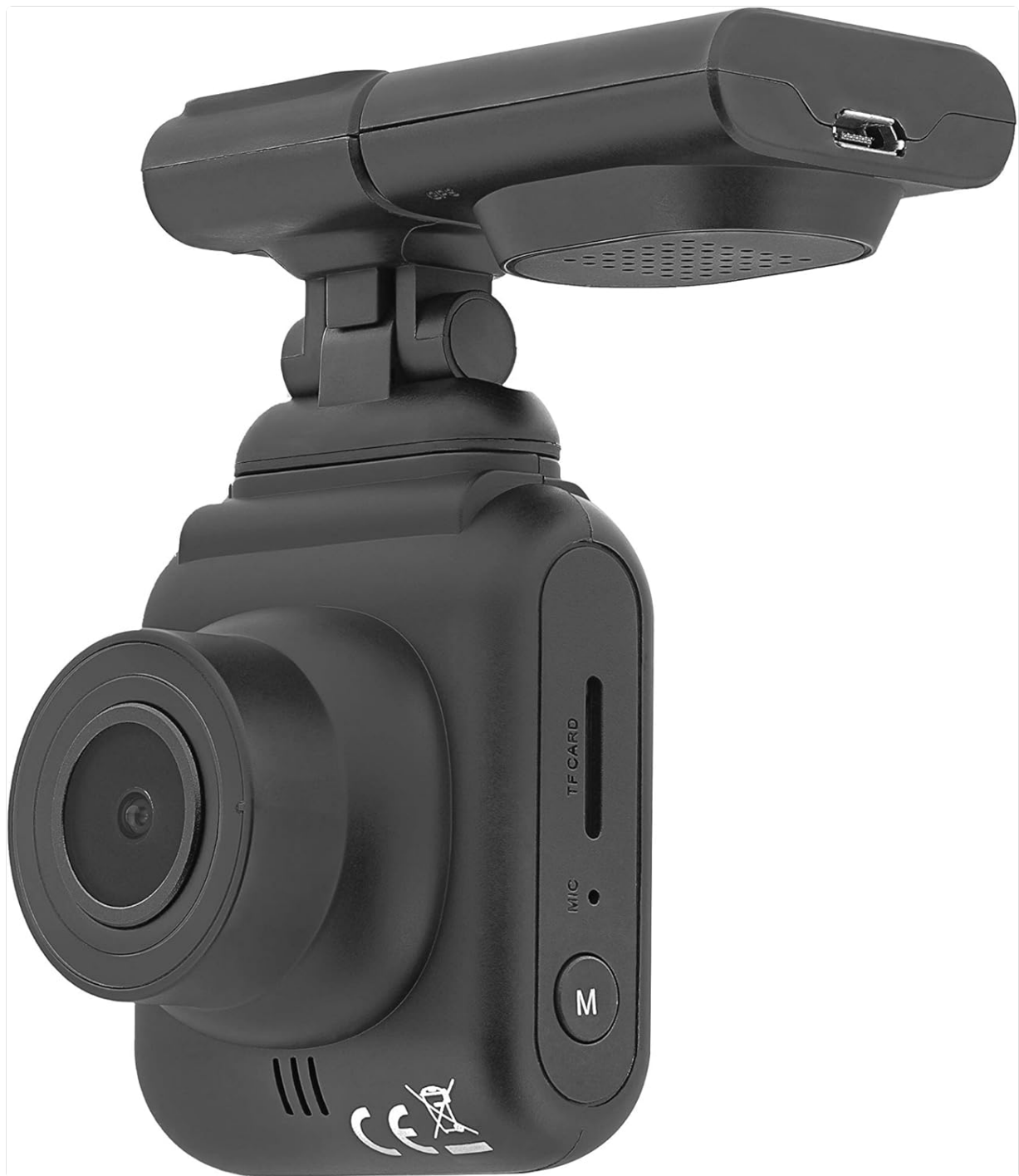
Image: Side view of the Dash Patrol DC2, showing the TF card slot, microphone, and 'M' button.
