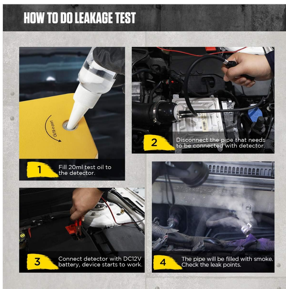
Figure 5.1: Filling Test Oil
