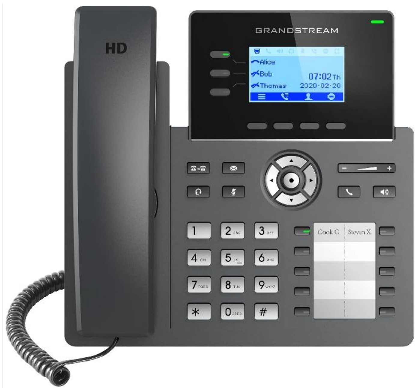
Figure 2.1: Front view of the Grandstream GRP2604P IP Phone, showing the display, keypad, and function buttons.
