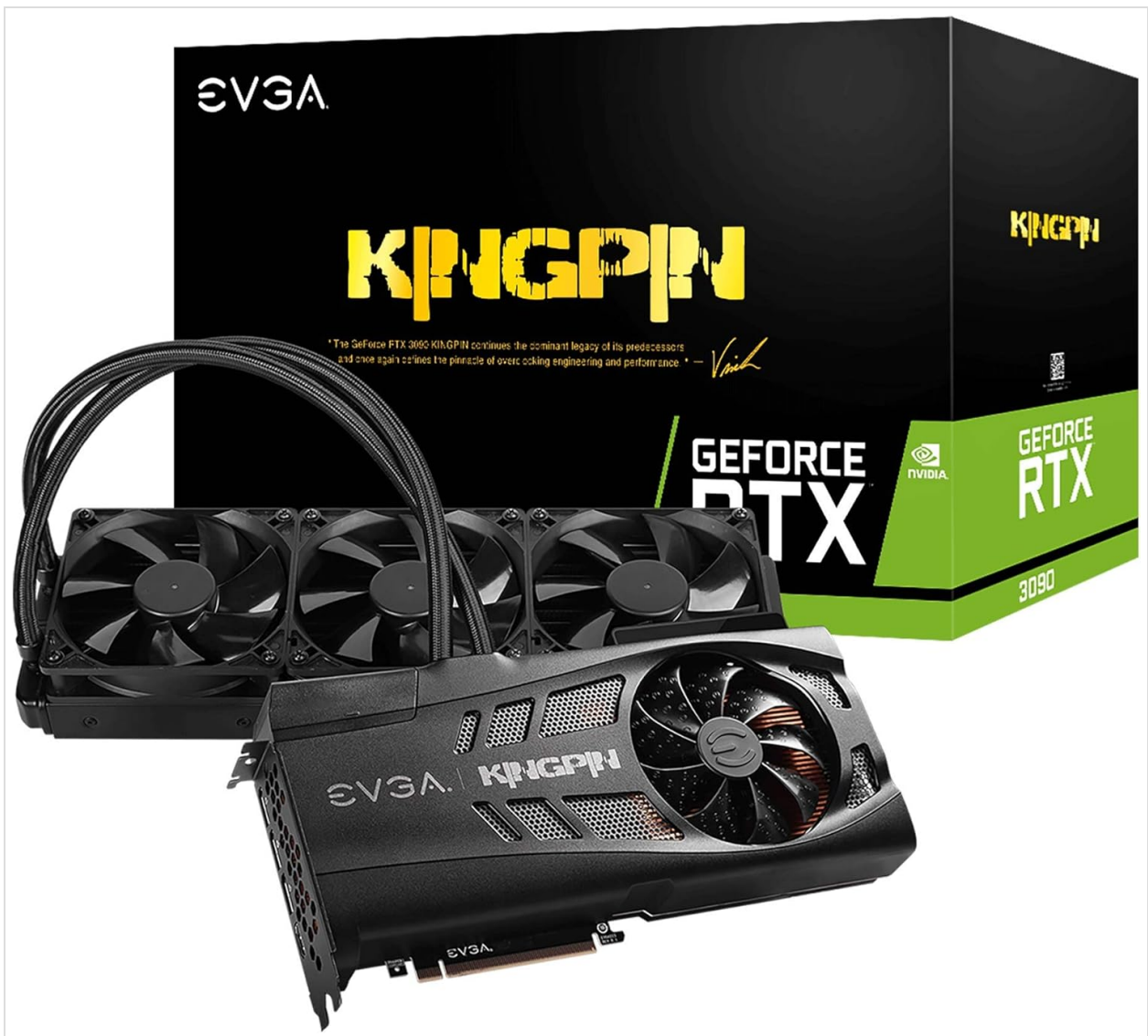
Image 1.1: The EVGA GeForce RTX 3090 K|NGP|N Hybrid Graphics Card shown with its retail packaging, highlighting the card's design and the included 360mm radiator.
